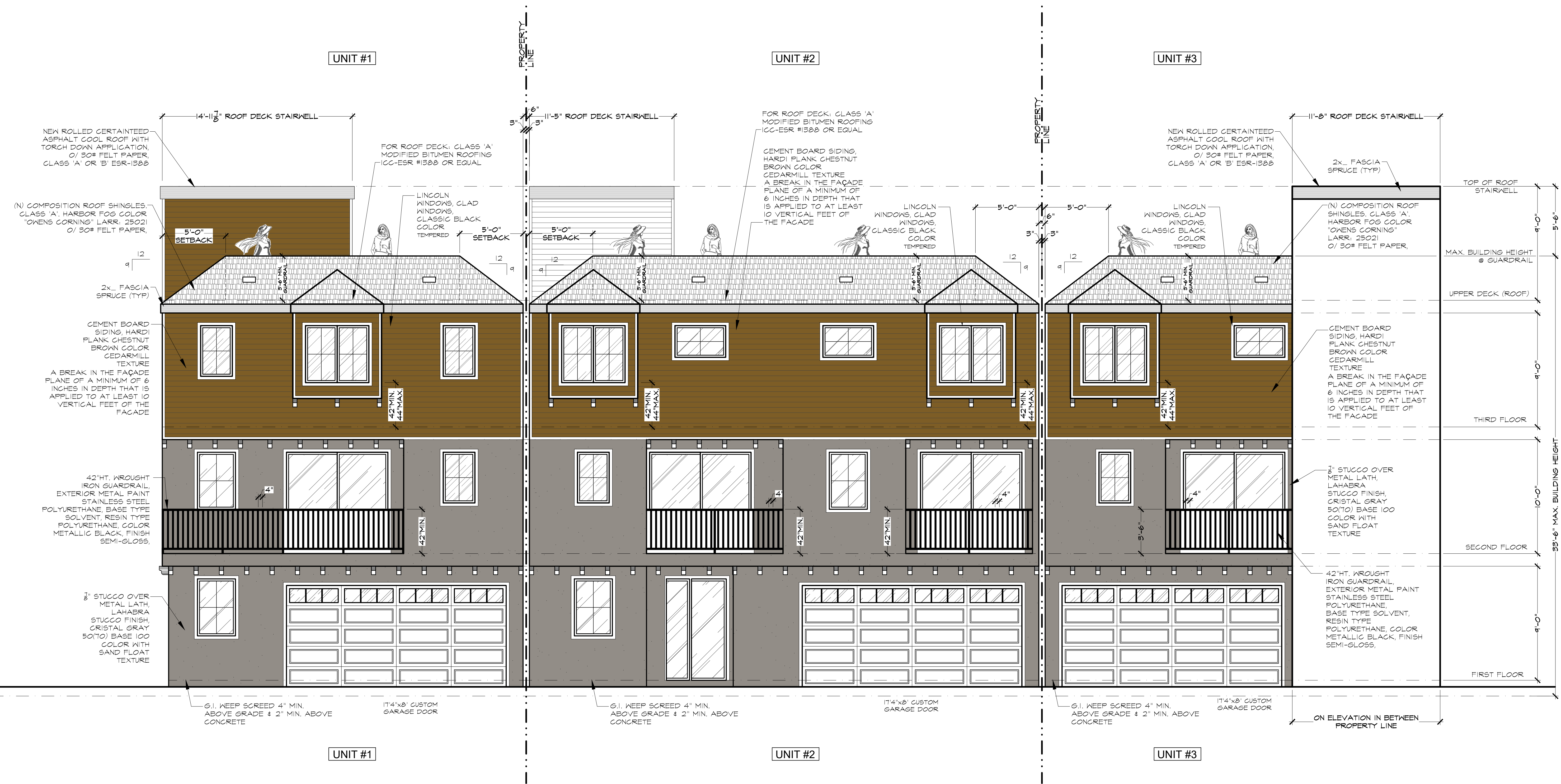
EAST ELEVATION - GARAGE DOOR SCALE: 1/4" = 1'-0"
