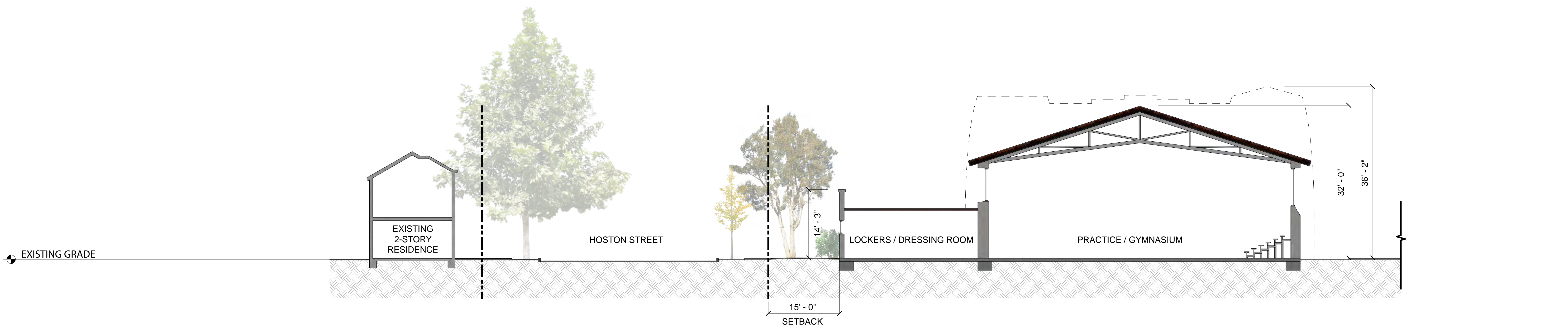
BLDG 4. PRACTICE GYMNASIUM BUILDING SECTION SCALE: 3/32"=1' 3
