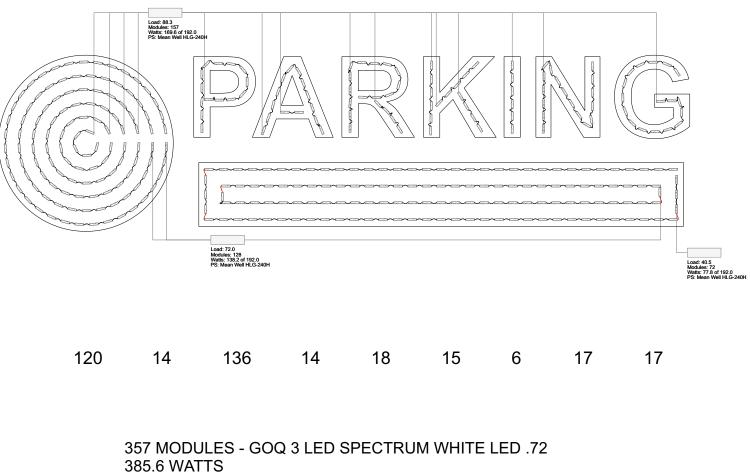
385.6 WATTS 1 POWER SUPPLY: HLG-240H-12 POWER SUPPLY MEAN WELL 4.0 AMPS
