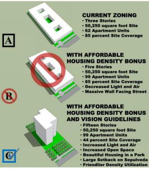
Figure 8. Panel A Shows a Building Under Current Zoning and Panel B Under a Density Bonus, While Panel C Shows an Alternate High-Rise Concept with Maximum Open Space
