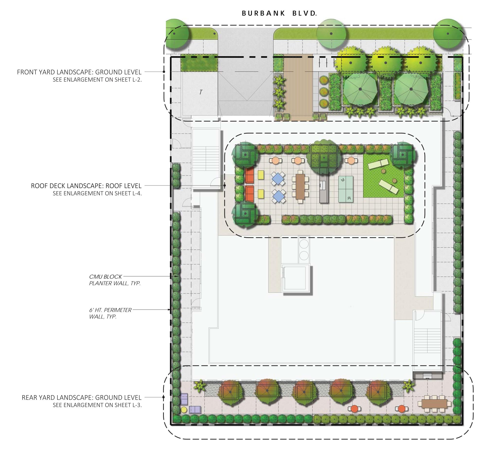
TREE COUNT SUMMARY TOTAL NO. OF UNITS PROPOSED = 55 TOTAL NO. OF TREES REQUIRED = 14 (1-24" BOX TREE PER 4 UNITS) NO. OF 24" BOX TREES PROPOSED ON GROUND LEVEL = 10 NO. OF 24" BOX TREES PROPOSED ON ROOF DECK = 4 TOTAL NO. OF 24" BOX TREES PROPOSED = 14
