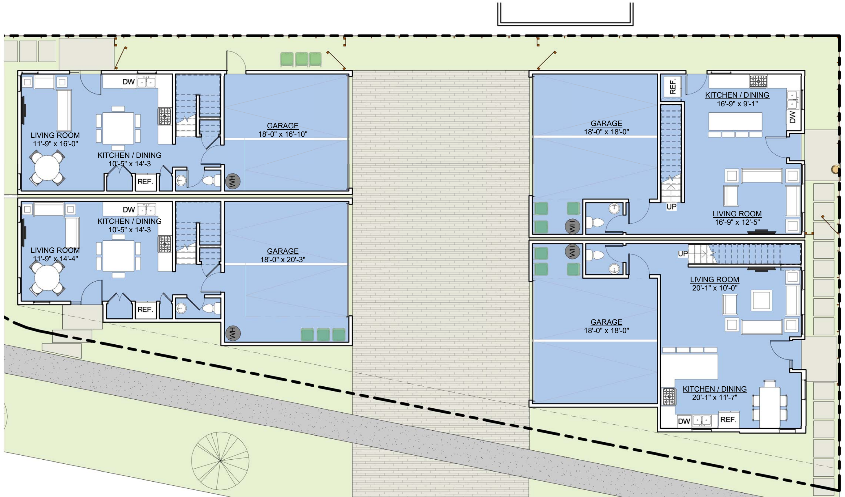
1 FIRST FLOOR PLAN 1/8" = 1'-0"
